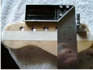
Mark on the masking tape the position of the securing screw hole, repeat process for other end hole. Joint the two securing hole marks, this should give you perfectly aligned tuning heads. If possible use a bench pillar drill to drill holes, I use a 1mm drill bit for screw depth and a 2mm drill bit one third depth to start the screw off. Be careful not to drill right through the headstock, it means a lot more work if you do. Take a break and have a cup of tea.
