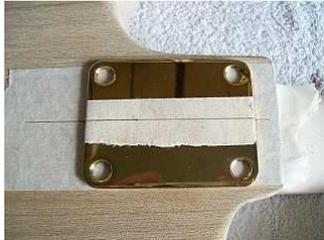
mark the centre of holes through neck plate , check the marks are square. Its difficult to get the neck and body into a drill press, so drilling holes by hand is the only answer. Clamp down neck and
