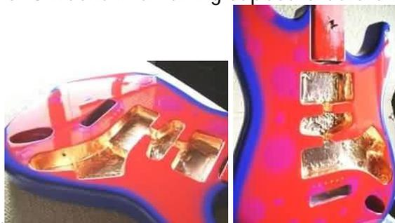
These two photos show the finished body with copper shielding in place.
