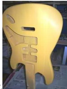
means you spray where you want to spray. The filler primer that comes with the PFkit works for two reasons, 1, primes ready for top coat, 2, the filler part gives you a bit of meat to rub down without going into the sealer.
