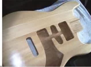
Once dry (see photo) it has a shiny finish. Using 1200 wet n dry, lightly sand over the PVA, this dulls the surface and gives a key along with its adhesive quality for the primer. When your satisfied the body is complete sealed, have a break and a cup of tea. You might have guessed by now I'm a great fan of tea breaks.
